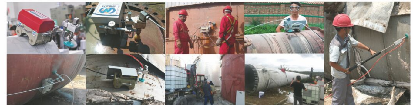
海德便携式水切割行走工装方案 HEAD brand portable water jet-cutting car solution
