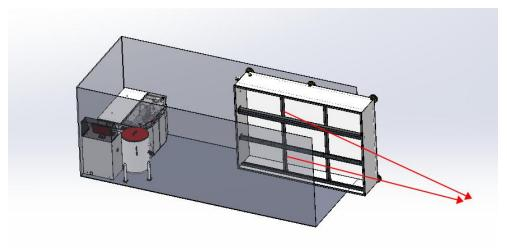
If the container is not moved to the bottom, two forklifts are needed to assist. One forklift pulls the entire water tank backward, and the other forklift forks the middle part of the water tank, and fixes the middle part of the water tank on the horizontally arranged forklift through a sling. A forklift is deployed to unload the water tank out of the container.
